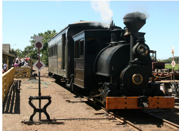
1890 Tank Porter Engine 'Cortez Mining Co #1'
